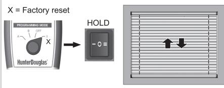
Press and hold I or II until the blind moves (for 5 seconds)
